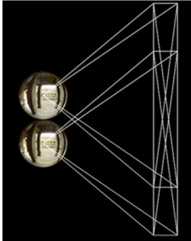
Fig 6: Position of cameras inside the panoramas and the projected views to a single screen. Note The Virtual Room has 8 screens and a different slice of the image appears on each screen to make up the whole panorama around all 8 screens.
